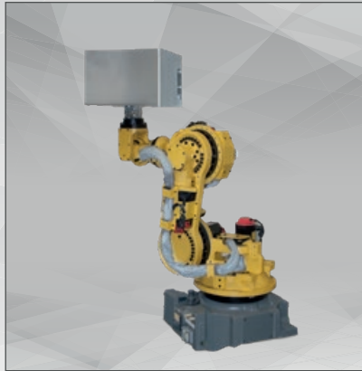
6-Axis-Shortarm-Robot for automated Grinding and Handling of rounded Parts
