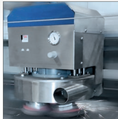
Triple Brush-Planetary Head for Deburring and Rounding
