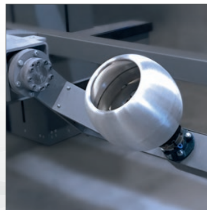
Turning device for Processing rotationally symmetrical workpieces
